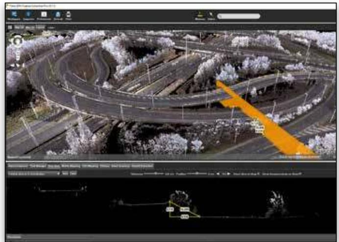
*Orbit 3DM Feature Extraction allows you to efficiently measure, extract, and detect assets. You can process cross-sections along the trajectory, create a profile along a 3D path, calculate mapping data and analyze volumes over time, export views and features, and create accurate reports.*
