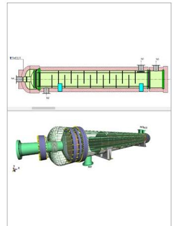
*Designs for an AES type heat exchanger.*
