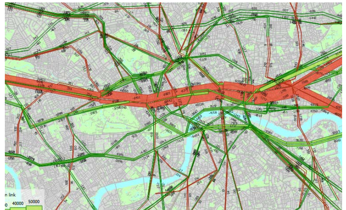
Change in a.m. peak period passenger volumes due to the Elizabeth Line.
