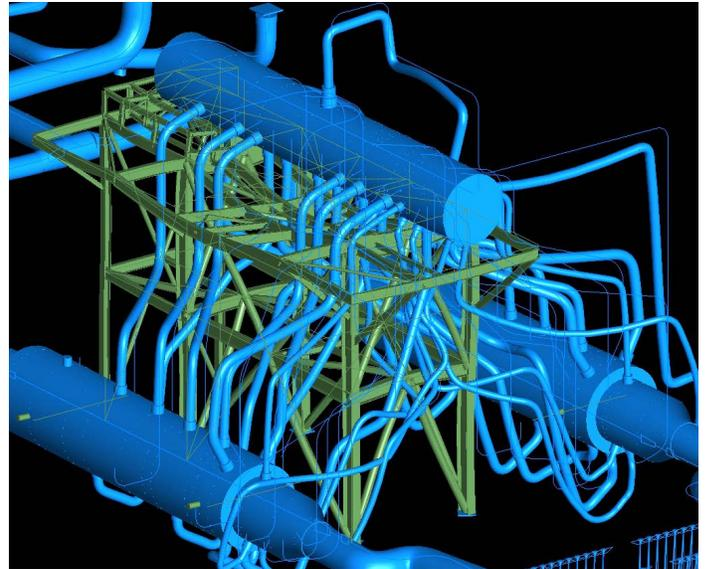
*Piping and framework models allow a more accurate understanding of the behavior of frameworks that are connected to piping supports.*
